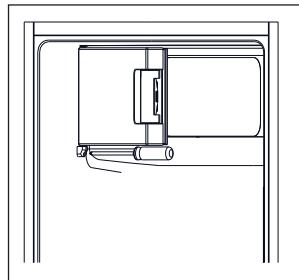
8. Unscrew bottom hinge. Then remove the adjustable feet from both side.
