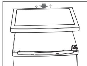
3. Unscrew top hinge and then remove door and place it on a soft pad to avoid scratch.
