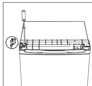
13. Put the top cover and fix it with 2 screws on the back.
