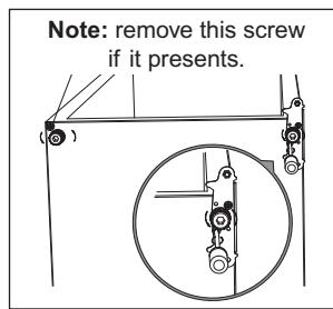
9. Unscrew and remove the bottom hinge pin, turn the bracket over and replace it.
