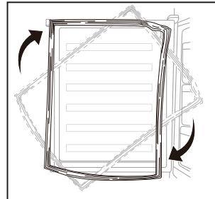
12. Place the door back on. Ensure the door is aligned horizontally and vertically, so that the seals are closed on all sides before finally tightening the top hinge.
