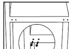
7. Lie down the rear of cabinet on a soft pad. And unscrew the bottom hinge and leveling foot.
