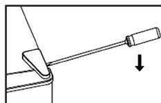
2. Unscrew the top hinge with a philips screw driver.
