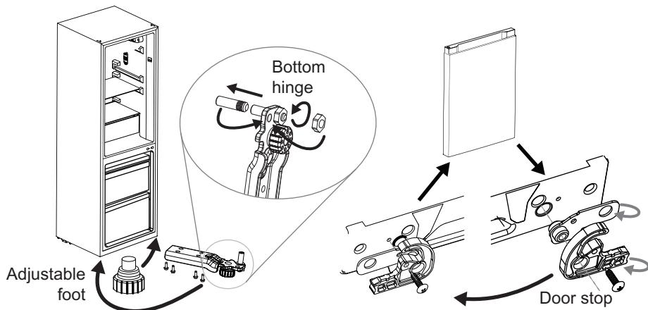
6. Put the freezer door on bottom hinge, install the middle hinge and the screw hole caps. Place the spacer on the upper axis of the hinge.
