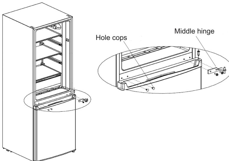
4. Dismantle the freezer door, the bottom hinge and adjustable foot of the other side.
