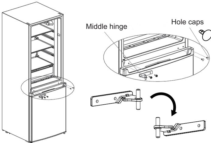
7. Put the refrigerating door on the middle hinge, install the upper hinge,upper hinge cover and hole cap on the other side.
