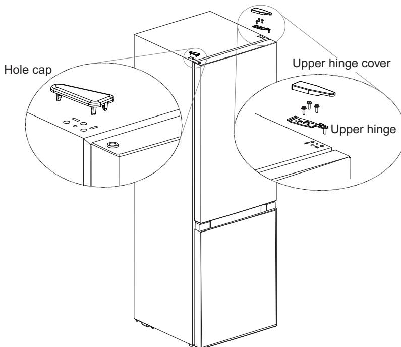
3. Dismantle the refrigerating door, the middle hinge, the screw hole caps.
