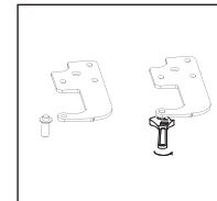
4. Move door switch from right hinge cover to left hinge cover in accessory bag.
