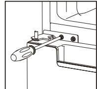
15. Replace upper door, please ensure the door align with the cabinet to make sure door gasket seal the cabinet tightly. Then connect door with cabinet by tightly fixed top hinge.
