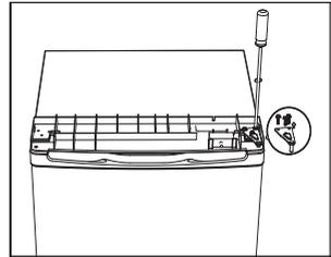
4. Unscrew bottom hinge of freezer door. Then remove the door and place it on a soft pad to avoid scratch.
