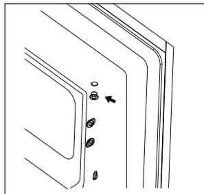
7. Rotate freezer door and place hinge side at left side.
