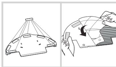
2. Open the rubber stopper **G1** and fill the mop attachment with water.
