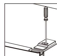
7. Take off the upper door, take out the screw from the middle hinge by cross screwdriver, then take off the lower door.
