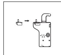
5. Detach cover in top of upper door and move harness from right side to left side, then replace the cover.
