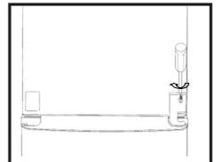
2. Unscrew and remove the hinge.
