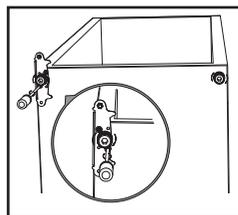
8. Make the middle hinge reverse the direction 180°, then transfer it to the left property position. Make the middle hinge pin in the upper hole of the lower door, then tight the bolts.
