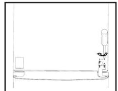
3. Unscrew middle hinge. Then lift lower door and place it on a soft pad to avoid scratch.
