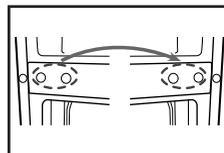
5. Unscrew bottom hinge. Then remove the adjustable feet from both side.
