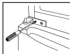
9. Place the upper door back on. Ensure the door is aligned horizontally and vertically so that the seal are closed on all sides before finally tightening the top hinge. Then insert the hinge and screw into the front of the unit.
