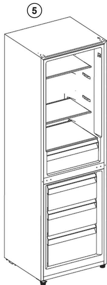
5. Take the freezer door, make sure the down hinge axis and the axis hole on the lower left side on the machine fix well and connect correctly. The freezer door is basically fixed now; then use the two screws to fix the middle hinge on the left side of the cabinet; then fix tight the middle hinge (as shown in the diagram No.6).
