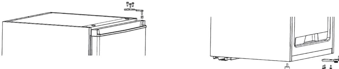
6) Fix the levelling feet bottom hinge in the opposite side.
