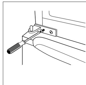
9. Unscrew the hinge pin and reverse the hinge, then reinstall the hinge pin.
