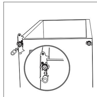
8. Make the middle hinge reverse the direction 180°, the transfer it to the left property position. Make the middle hinge pin in the upper hole of the lower door, then tight the bolts.
