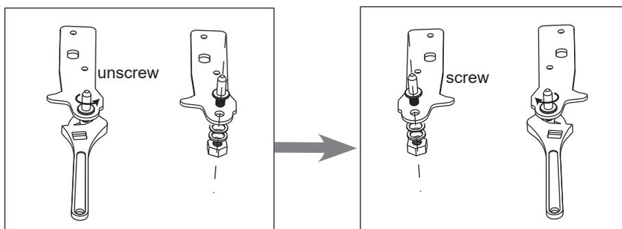
7. Refit the bracket fitting the bottom hinge pin. Replace both adjustable feet. Transfer the lower door to the property position..
