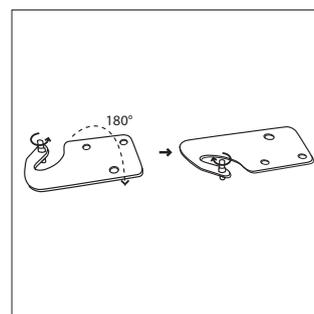
10. Place the upper door back on. Ensure the door is aligned horizontally and vertically so that the seal are closed on all sides before finally tightening the top hinge. Then inert the hinge and screw into the front of the unit.
