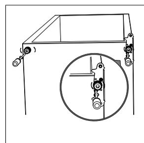
6. Unscrew and remove the bottom hinge pin, turn the bracket over and replace it.
