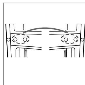
5. Unscrew bottom hinge. Then remove the adjustable feet from both side.
