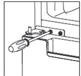
8. Place the upper dor back on. Ensure the door is aligned horizontally and vertically so that the seal are closed on all sides before finally tightening the top hinge. Then inert the top hinge and screw it to the top of unit and then fix hinge cover (in accessory bag) by screw.
