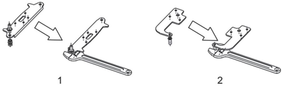
6. Install the lower hinge under to the refrigerator like below, screwing in the adjusting feet, make sure the position in horizon.
