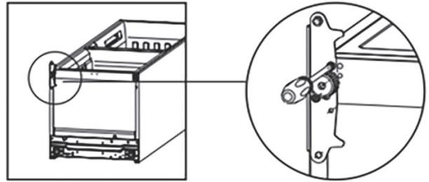
7. Install the lower door, adjust and fix the middle hinge onto the cabinet.
