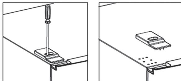
3. Take off the upper door, take out the screw from the middle hinge by cross screwdriver, then take off the lower door.
