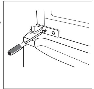
10. Place the upper door back on. Ensure the door is aligned horizontally and vertically, so that the seals are closed on all sides before finally tightening the top hinge.
