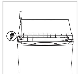
11. Put the top cover and fix it with 2 screws on the back.
