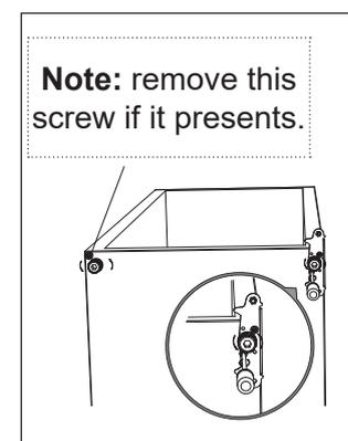
7. Unscrew and remove the bottom hinge pin, turn the bracket over and replace it.
