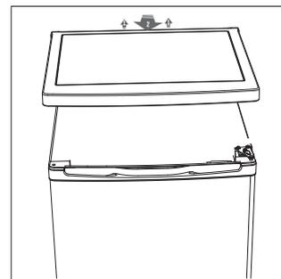
3. Unscrew top hinge and then remove upper door and place it on a soft pad to avoid scratch.
